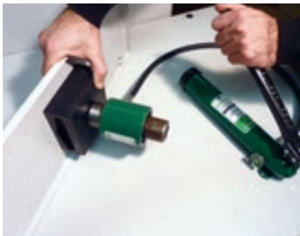
Making the cut-out with a punch.
